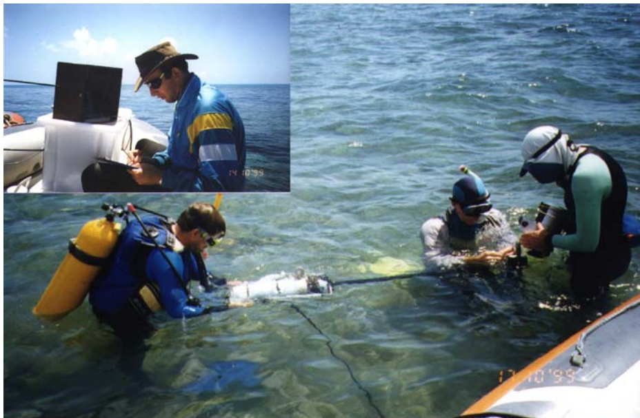
Figure 3.5.1: Attaching video camera to sensor head of the underwater hyperspectral radiometer.
