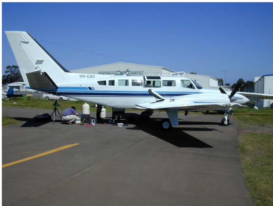
Figure 4.2.3 Cross-calibrating ground based instruments with HyMap™ on board its aircraft platform.
