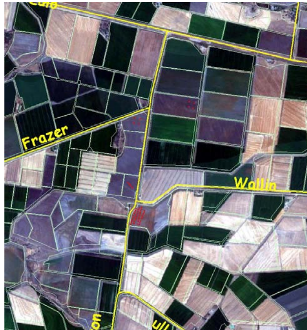
Figure 4.2.4: Detail of Figure 4.2.1 showing co-registration with GIS strings. This was made as part of the Coleambally information system using HyVista provided information.
