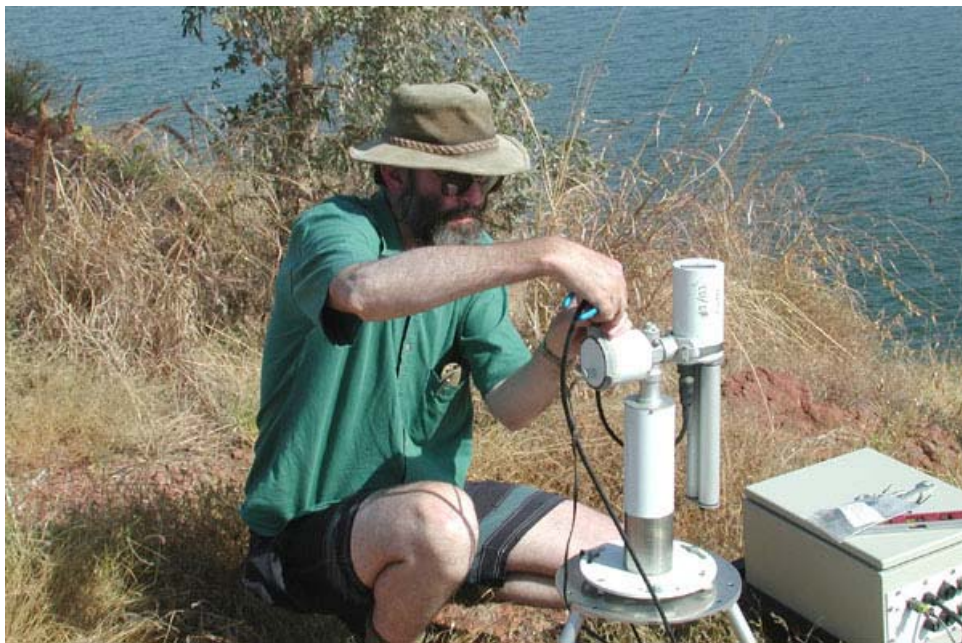
Figure 2.4.1 CIMEL being serviced at Lake Argyle during field campaign
