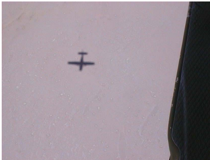
Figure 2.2.3: Lack of “hotspot” halo around aircraft shadow indicates flat smooth but diffuse texture. However, there is a pattern of “mottles” to take into account.
